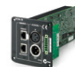
RCM-28 OMNEO Network and DSP Module for Tour Grade Amplifiers
