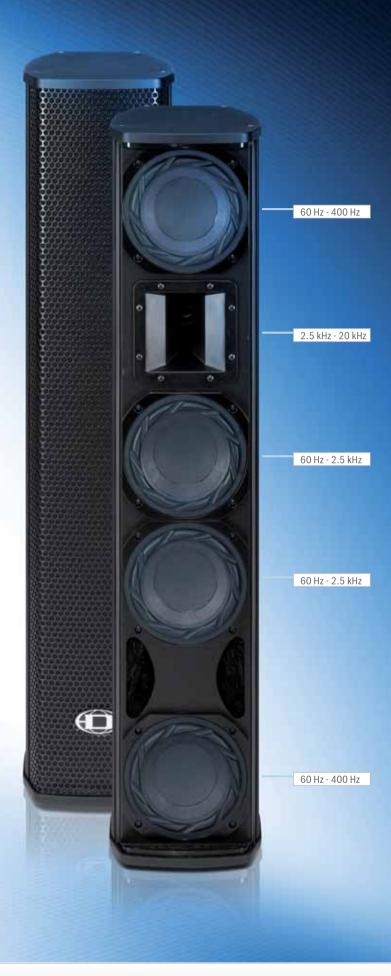
The TS 400 is equipped with 4 x 6,5" DND 6130-16 Neodymium woofers and one Electro-Voice DH3 compression driver coupled with a 90° by 40° constant directivity horn providing very high SPL and excellent coverage. Power handling is 600W RMS / 2.400W peak.
