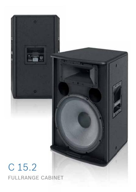
In the C 15.2, DYNACORD is offering an extremely compact, trapezoidal 15" / two-way full-range cabinet boasting very good power handling (500W continuous / 2000W peak) and sensitity of 100 dB 1W / 1m for applications requiring an extended low end.
