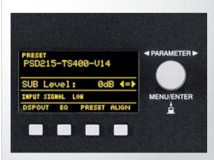
The integrated 24-bit digital controller with internal 48-bit double-precision resolution exhibits a 1-into-3 topology: SUB channel, TOP channel and an additional DSP Out.
